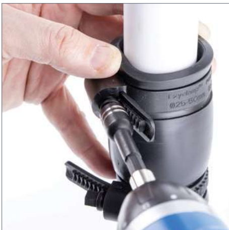
Tighten using Electric Screw Driver
