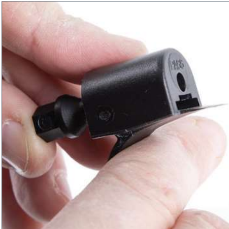
Insert Screw into Housing
