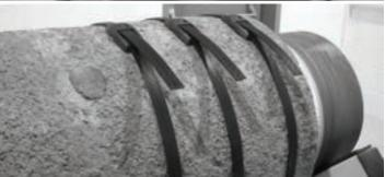
Tests have been carried out fitting various Smart® Band product to concrete coated pipe. This was to determine if the abrasive surface of the concrete pipe had an adverse effect to the product during fitting.
