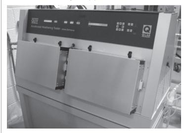
The QUV accelerated weathering tester simulates outdoor conditions by subjecting the test pieces to UV light and moisture in alternating sequences at elevated temperatures. Tests are carried out in line with appropriate international standards where applicable.
